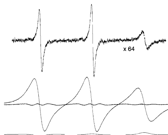
Figure 3. EPR spectra due to 0.1 (top trace, at a relative gain of \times 64 ) and 93.6 mM (middle trace) PDT in 70% glycerol at 273 K. The fit and spectrum are indistinguishable; however, a definite residual is evident. Furthermore V_{\text{disp}}^{\text{obs}}(+1) < 0 and V_{\text{disp}}^{\text{obs}}(-1) > 0 the reverse of the signs expected from exchange. The contribution of exchange is negligible, \Omega(T) = 0.006 \pm 0.018 .
